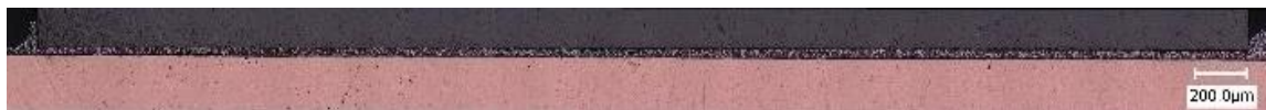
Fig.3 Cross section of the sample bonded by Ni nanoparticle/Al particle composite paste
