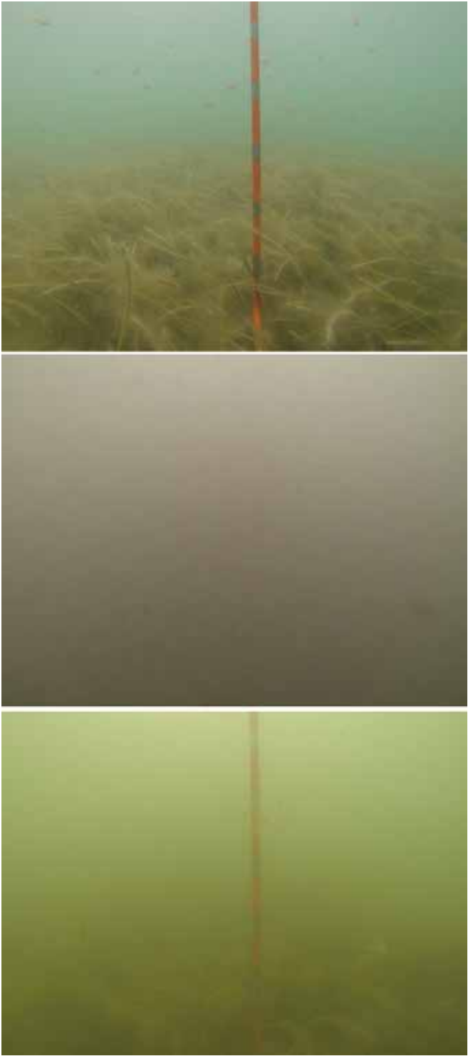
Figure 4. Underwater photos of turbidity increase and decrease during the dredging operation. Upper: Condition before the dredging operation; the dense seagrass extends about 20 cm from the seabed. Middle: Condition at the peak of the dredge turbidity plume; the reference rod about 0.5 m in front of the camera has become invisible. Lower: Condition 50 minutes after the turbidity peak; the visibility has recovered considerably.
