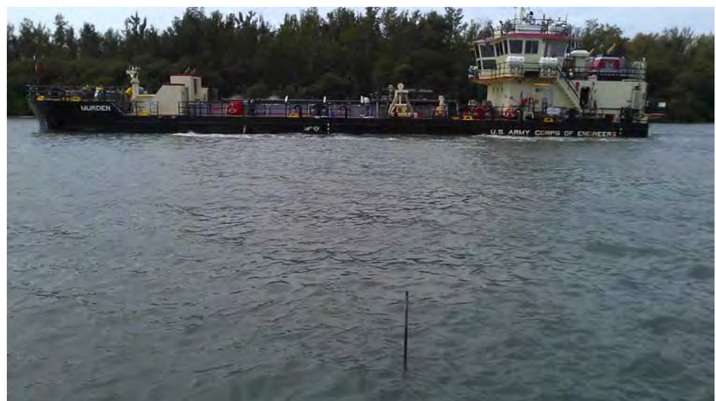
Figure 2. The USACE special operations hopper dredge, Murden, passing in front of the measurement site (metal pole at the bottom of the picture). The slurry was pumped into the container of the dredge. The overflow is visible along the side of the vessel.
