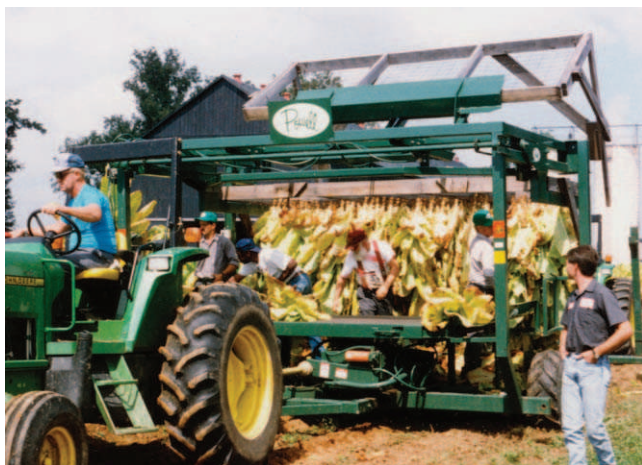
Figure 7. Powell harvester system for harvesting burley tobacco.
