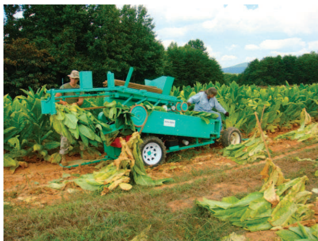
Figure 6. Burley Spiker stalk spearing machine.
