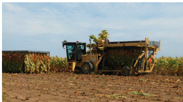
Figure 12. GCH automated harvester for burley tobacco.
