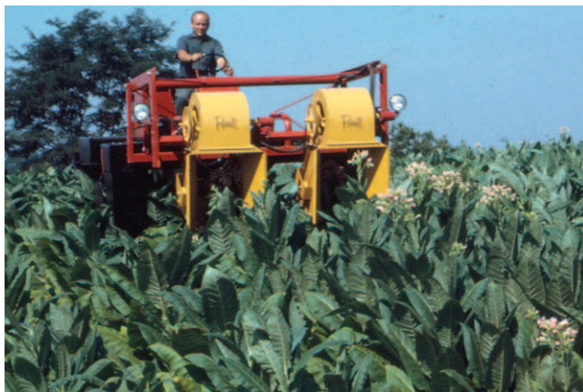
Figure 3. Mechanical topping of burley tobacco.
