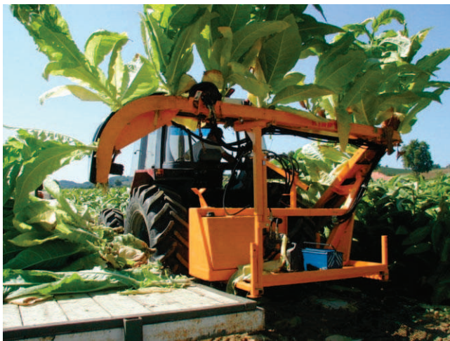
Figure 9. Kirpy notching-type harvester for burley tobacco.
