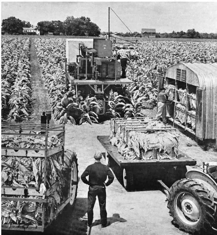
**Figure 9.** Picture from a Powell Manufacturing Company ad from about 1968 showing their prototype mechanical harvester and commercial bulk curing barn.
