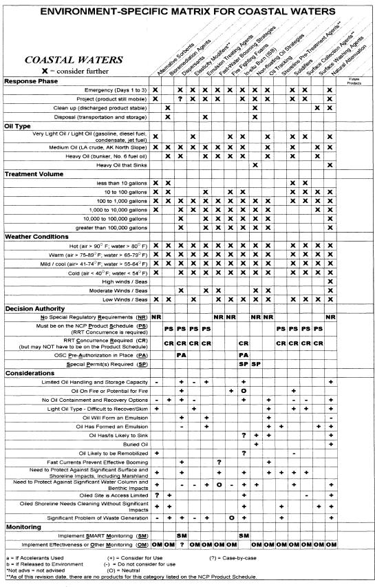
Figure 1. Environment-specific matrix for coastal waters. This is one of three environment-specific matrices contained in the Selection Guide. The other two matrices cover oil on inland waters and on land.
