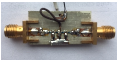
Figure 5: Fabricated NLTL with periodically arranged varactor diodes and inductors.
