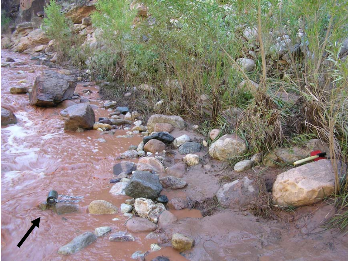
Figure 3. Photograph of Shinumo Creek looking upstream near the confluence with the Colorado River. The Onset StowAway XT132 temperature logger (lower left in photo) is inside a plastic case inserted into a piece of steel pipe. The instrument is tethered to a tree on shore using chain and coated steel cable.
