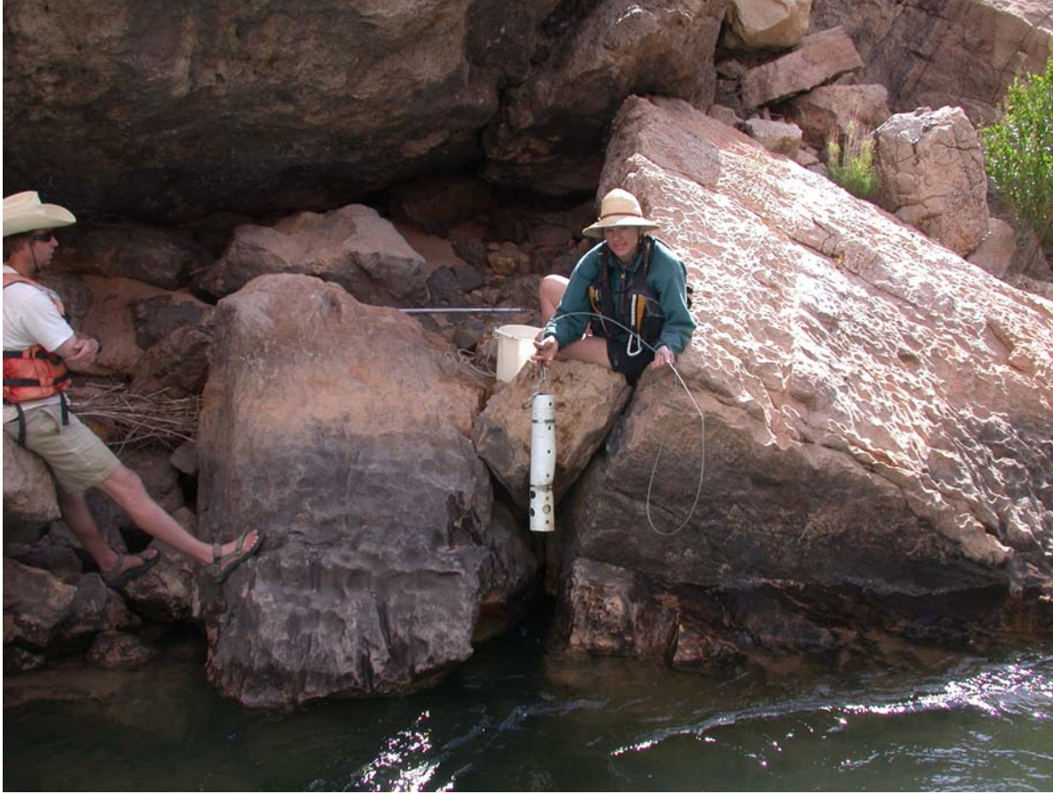
Figure 4. Photograph of the east bank of the Colorado River near river mile 61. The Yellow Springs Instruments multiparameter instrument shown in the center of the photograph is protected from abrasion inside of a perforated plastic sleeve and deployed in the river using coated steel cable.
