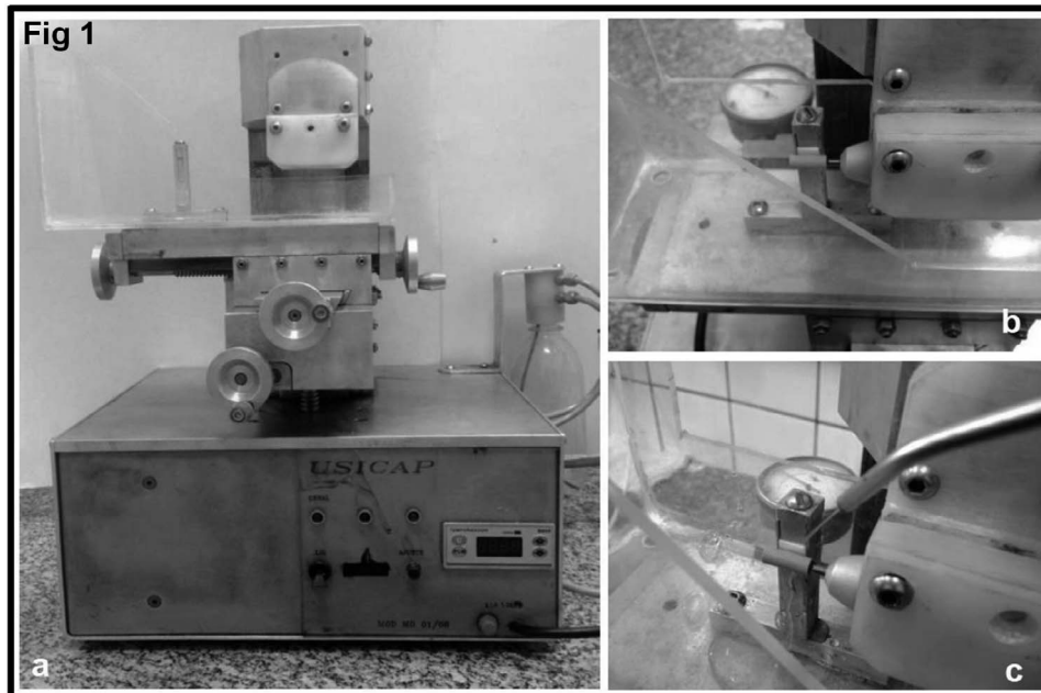
Figure 1. (a): Grinding device. (b): Dry grinding. (c): Wet grinding.
